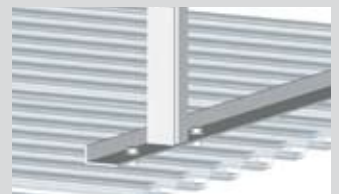
Foil roof with gravel filling: Fastening to framed panels and loading with gravel
