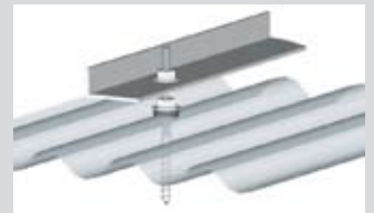
Corrugated fibre cement roof: Attaching with hanger bolts
