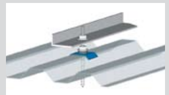
Trapezoidal sheet roof: Attaching with hanger bolts
